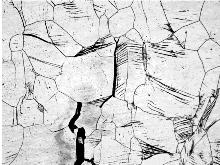
Figure 4. SIPH, deformation twins, intergranular cracking, 200x
